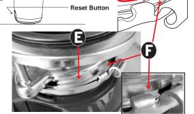
As the Lower Mount Ring is turned counter clockwise each tab slides up onto the Upper Mount Ring Ramp (E) and locks in position <u>over</u> the Ridges (F).
