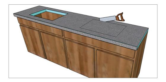
Cut out for the sink using a jigsaw or handsaw. As needed, recess cuts might be created with a utility knife or a router to accommodate recessed sinks. Cutting the holes may proceed before or after installation of large format, thin porcelain tile as indicated in step 05.
