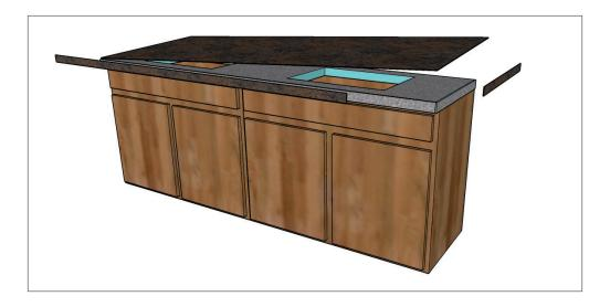
O4 Install the large, or small format tile, including thin veneer tile, or stone to the wedi Building Panel surface and edges using a modified thinset.
