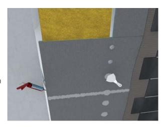
structurally sound and service condition acclimated ( wood) and cured ( concrete) substrates. Excessive movement may be tolerated initially as long as the substrate regains its original setting ( no excessive permanent settling can be protected against). The wedi Joint Sealant is of high viscosity and exhibits excellent non-sag properties.
